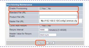
Step 3. Phone get Master File from provisioning server from address input into WEB setting.
