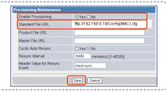
Step 3. Phone get Standard File from provisioning server from address input into WEB setting.
