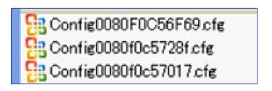
Config{MAC}.cfg: for each unit setting file like account name, password and SIP Server address.
