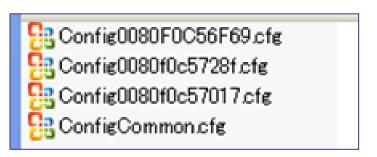
ConfigCommon.cfg: for common setting across all phones, like SIP server address.
