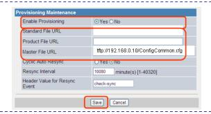
Step 3. Phone get Master File from provisioning server from address input into WEB setting. And then, Phone get Product / Standard File from provisioning server by using address described in Master File.
