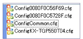
ConfigCommon.cfg: for common setting across all phones, like SIP server address.
