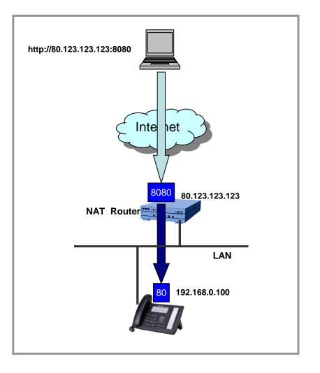
**Port forwarding** are well-known technologies for enabling internet remote access to local devices behind NAT router or firewall.
