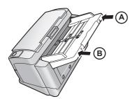
(3) Pull out the feed tray extension in the direction of the arrow shown in the illustration below.
