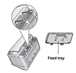
• When using the mixed batch card guide, install it in the reverse order of uninstallation. For details on the mixed batch card guide, refer to the Operating Instructions.
