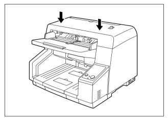
**8.** Connect the power cord and the USB cable to the scanner.
