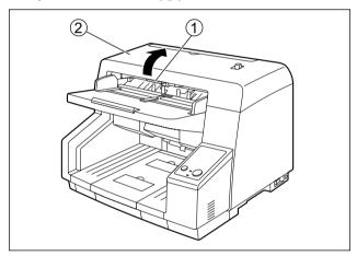
**4.** Pull towards you and remove the double feed prevention roller cover by using the indent (①).
