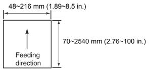
Paper thickness:  $40\sim209 \text{ g/m}^2 (11\sim55 \text{ lb.})$ The height of all the documents on the tray should be less than 5 mm (0.2 in.). This compares to 50 sheets (80 g/m<sup>2</sup> or 20 lb.) of new paper.
