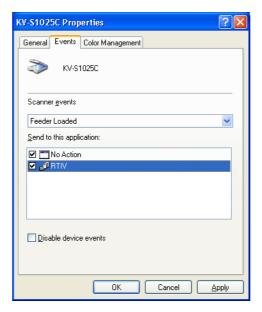
• To disable the automatic activation of the scanner applications, set the [Disable device events] check box to on.
