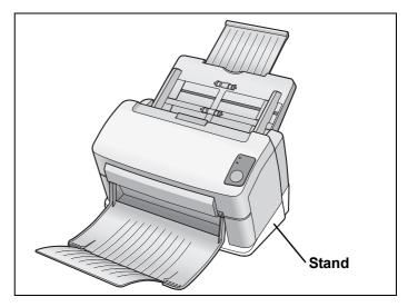
Place the scanner on an even surface as shown in the illustration, and then loosen the two screws counterclockwise.
