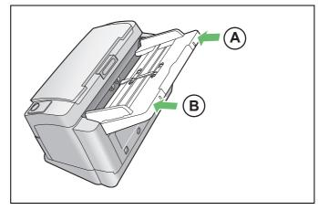
Pull out the feed tray extension in the direction of the arrow shown in the illustration.
