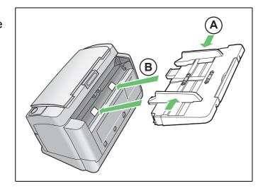
Push the right ( A ) and left ( B ) sides of the feed tray in that order until the feed tray locks in place.
