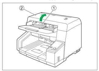
3. Use the roller cleaning paper (page 51) to remove the dirt from the surfaces of all rollers.
