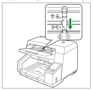
**9.** Place the document on the hopper again and adjust the document guide according to the size of the document to be scanned.
