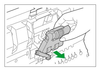
4. Take out the new paper feed roller module in the optional "Roller exchange kit (KV-SS039)".
