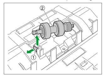
5. Take out the new double feed prevention roller in the optional "Roller exchange kit (KV-SS039)".
