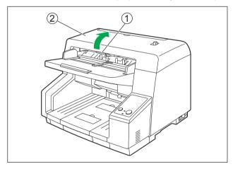
**3.** Pull towards you and remove the double feed prevention roller cover by using the indent (1).
