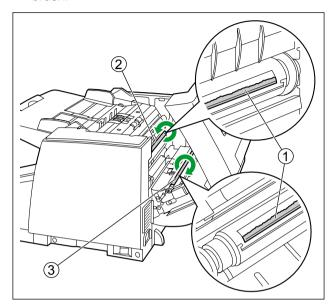
• After cleaning, rotate the reference plates (②, ③) in the directions indicated by the arrows to return the plates to the original background color.
