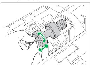
7. Insert the protrusion (①) of the double feed prevention roller cover into the hole on the main unit, and then push in the part of the roller cover indicated by ② in the direction indicated by the arrow until it clicks into place.
