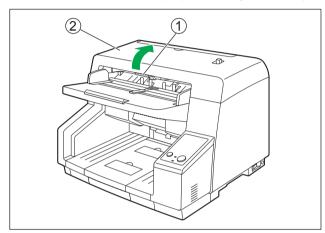
**3.** With a dry cloth, wipe off any dirt on the conveyor (①).
