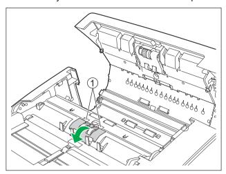
**4.** While pulling the tab (①) in the direction indicated by the arrow, lift the double feed prevention roller (②) in the direction of the arrow. Then, pull out the right shaft (when facing it) from the notch in the roller mount.
