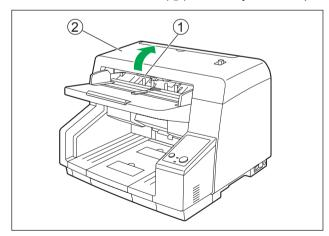
**3.** Move the lever (①) of the paper feed roller module in the order indicated by the arrow (①, ②), and then pull out the module towards you.
